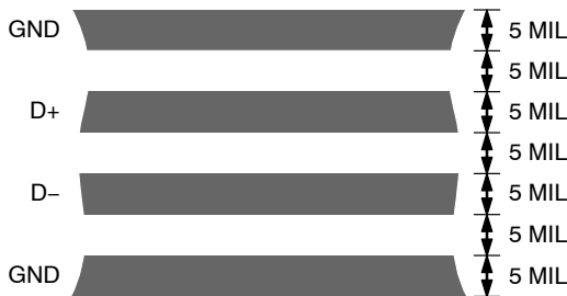
Figure 22. Typical Arrangement of Signal Tracks
